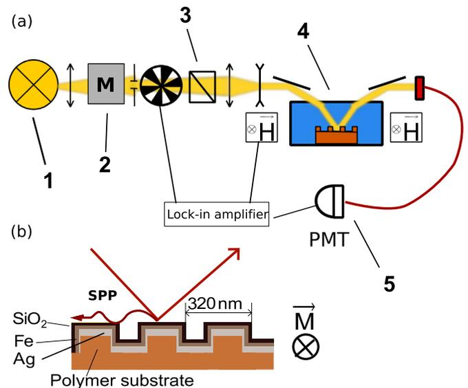
Fig. 1. (a) The scheme of the experimental setup for the magneto-optical surface plasmon resonance sensor: 1 – light source, 2 – monochromator, 3 – Glan-Taylor prism, 4 – flow cell with magnetoplasmonic crystal in an alternating magnetic field, and 5 – photomultiplier tube. (b) The scheme of the magnetoplasmonic trilayer structure and excitation of surface plasmon polaritons.
