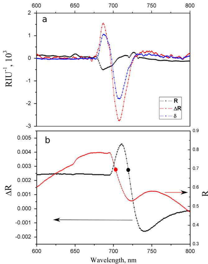
**Fig. 4.** (a) Spectral dependences of MOSPR sensor sensitivity calculated from experimental spectra for different modes of detection. (b) Maximum sensitivity points for different modes of operation in reflectance and  $\Delta R$  spectra.
