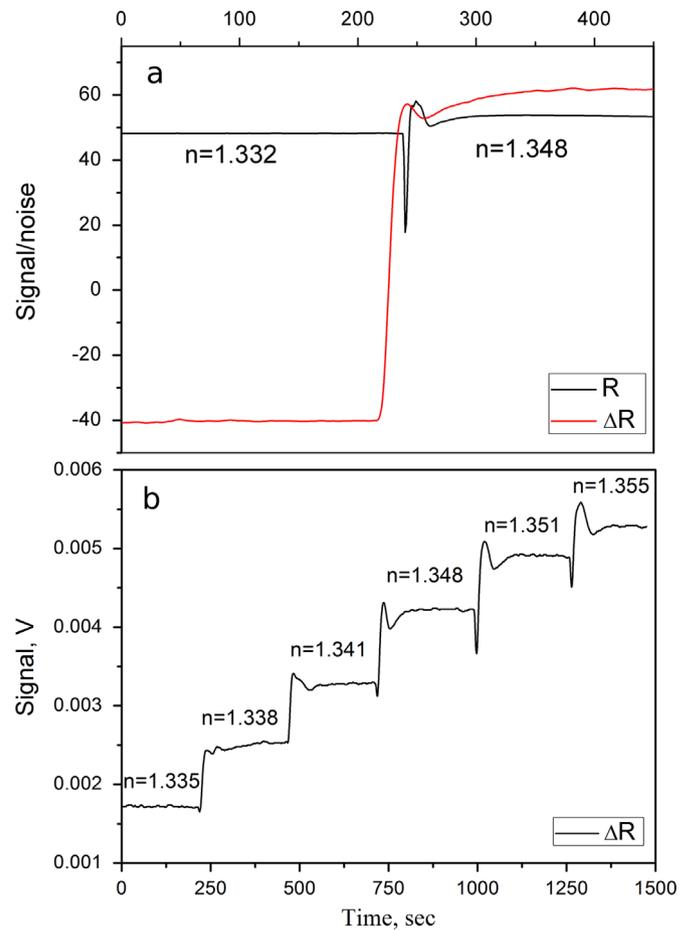
**Fig. 5.** (a) Signal/noise time dependence of the MOSPR sensor for the reflection and  $\Delta R$  modes of detection under varying liquid concentration in the flow cell. (b) The signal of the MOSPR sensor in the  $\Delta R$ -mode and real-time regime.
