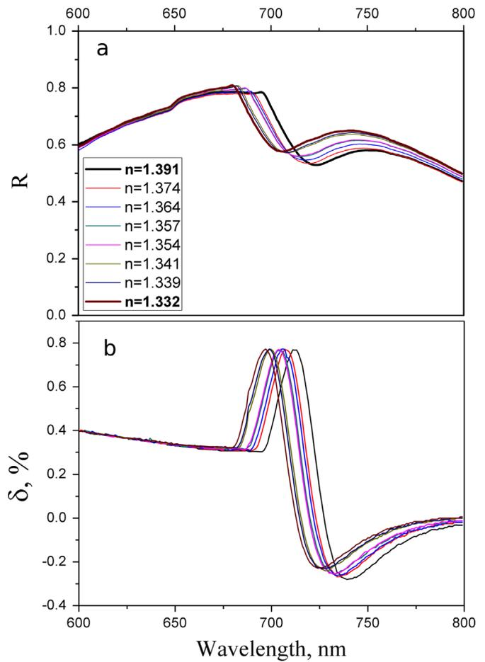
**Fig. 3.** The dependence of the reflectance (a) and TMOKE (b) spectra of the magnetoplasmonic crystal measured at an incident angle of  $55^\circ$  on the refractive index of liquid in the flow cell for the trilayer structure Ag(100 nm)/Fe(5 nm)/SiO<sub>2</sub>(10 nm).
