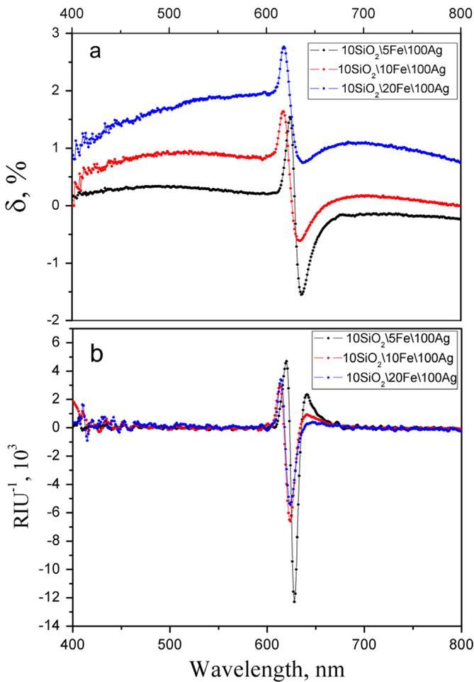
**Fig. 2.** (a) TMOKE spectra of magnetoplasmonic crystals with 5-, 10- and 20-nm Fe layers measured at an incident angle of  $68^\circ$  at the interface with air. (b) Sensitivity of MOSPR sensors calculated from the TMOKE spectra on (a) by using Eq. (7).
