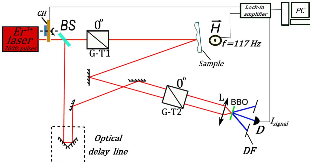
Fig.1. Experimental setup for measurements of second-order correlation functions. CH is a mechanical chopper, BS is a beam splitter, G-T1 and G-T2 are Glan-Taylor polarizers, L is a focusing lens, BBO is a nonlinear optical crystal, D is a detector, H denotes the external AC magnetic field, DF is an aperture.
